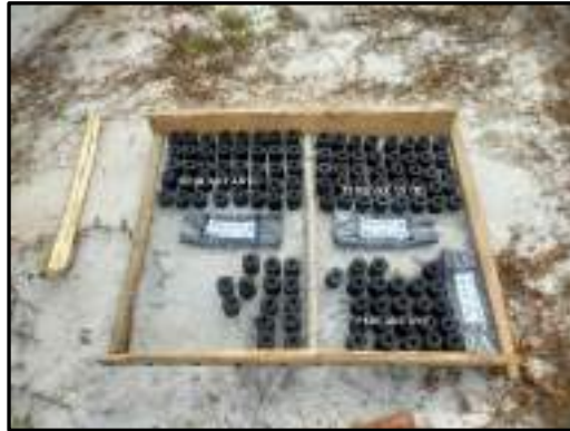
Gambar 4.22 Proses Penjemuran Briket Arang
